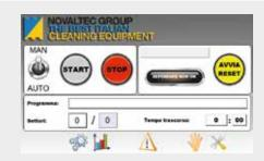
The automatic belt washer is equipped with a 7" contol panel to set belt functions such as belt lenght, speed, number of sector, etc..
